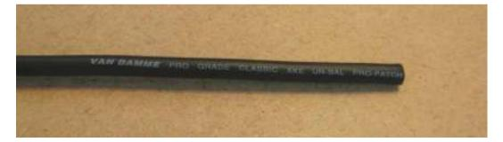
3. Strip about 1.5cm of the outer jacket, using a cable stripper or a utility knife. Make sure you don't cut too deep and harm the copper shielding.
