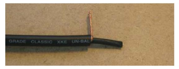
5. Gently remove the black carbon jacket close to the bare copper, and leave about 1-2mm.
