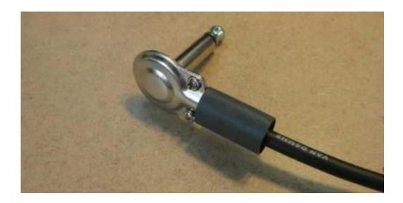
16. Use a heat gun to shrink the tubing. While keeping a distance of 20cm between the plug and the heat gun, rotate the plug slowly – allowing the tubing to shrink evenly on all sides. When you see the glue starting to melt, you can stop the heating. Put the cable aside to cool for few minutes.
